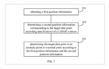
The patent introduces a novel method to enhance the reliability and security of LiDAR systems by detecting anomalies in point cloud data. It calculates an anomaly score based on the deviation of target data points from expected positions, allowing for efficient identification of potential attacks or malfunctions. The real-time nature of the calculations and its compatibility with existing systems make it a practical solution for improving the safety of vehicles equipped with LiDAR technology.
